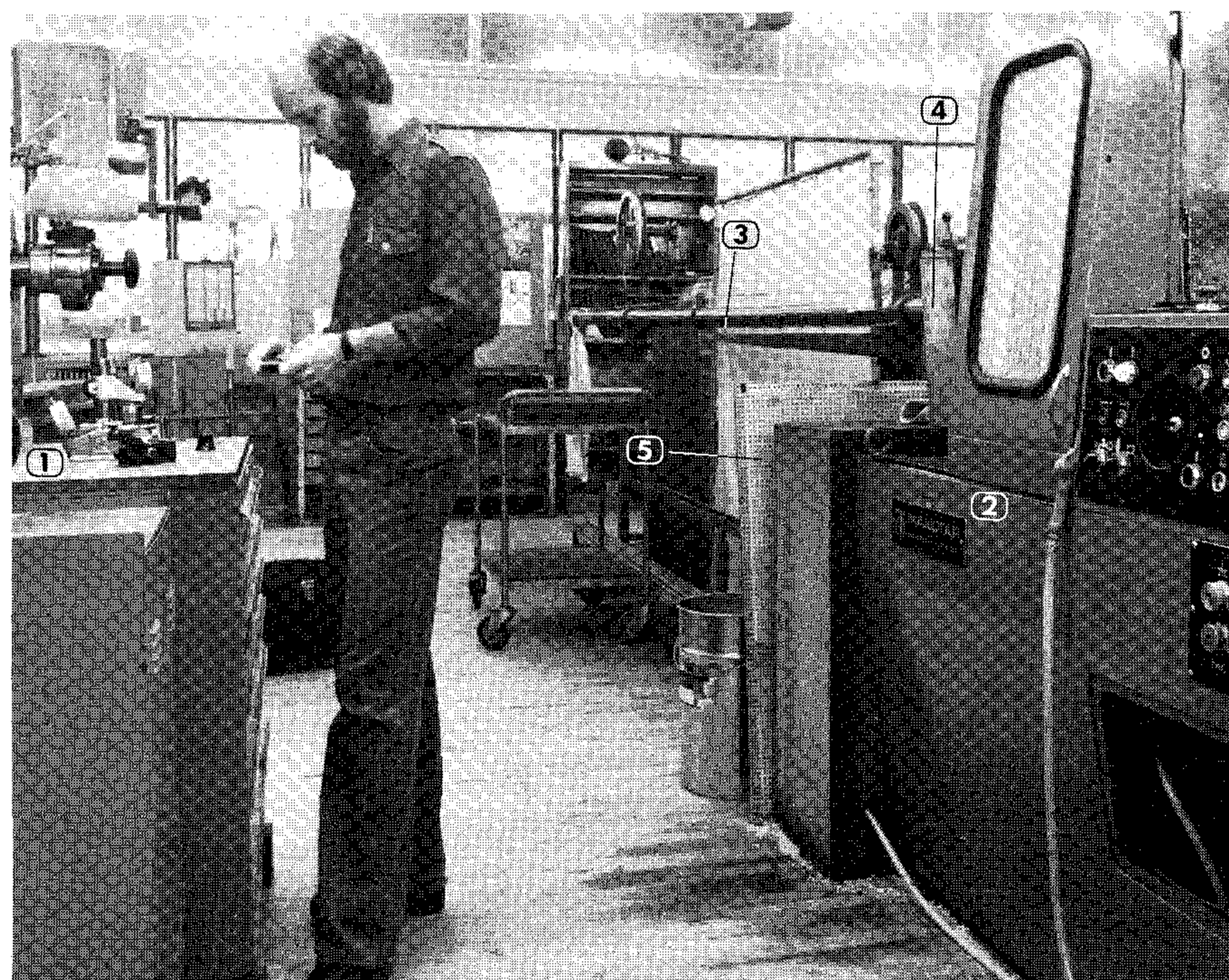
① Quality control bench ③ Feed-tube ⑤ Screen ② Lathe ④ Hood
